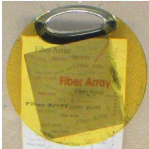
Figure 9: Image through a fiber array filled with a nonlinear material
