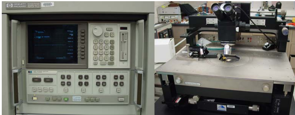
Fig 2. HP 8510 Network Analyzer and Cascade Microtech 11000 Probe Station
